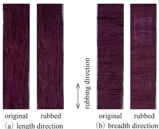
Fig. 5. the original sample and the sample rubbed to 500 times.
